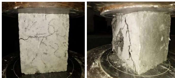
Fig:4.2. Compression testing
