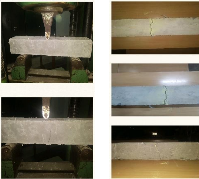
Fig:4.6. Flexural test on prism
