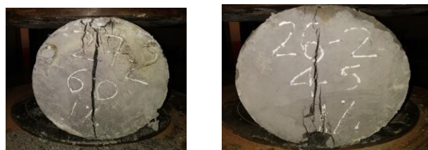
Fig:4.4. Split tension test
